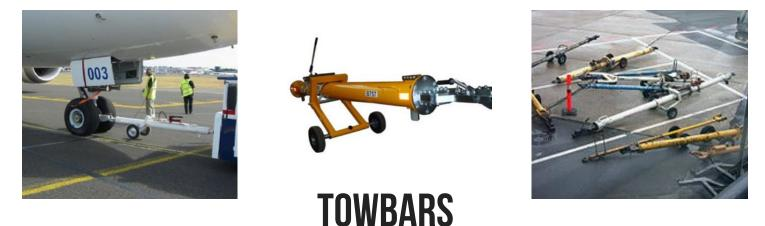
Conventional tugs use a tow bar to connect the tug to the nose landing gear of the aircraft.
